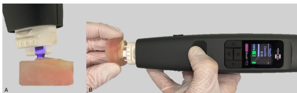
Fig. 2 A/B Application of dielectric barrier discharge plasma with a handheld device (piezobrush PZ3, Relyon Plasma, Regensburg, Germany). Close up image of the plasma electric discharge on the enamel
