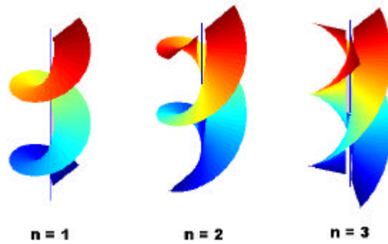
FIGURE 5.4 The helical wavefronts of the optical vortices with n = 1 , n = 2 , and n = 3
